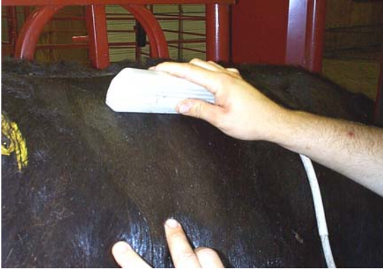
Reference 1. The technician is collecting the across image shown on the right for calculation of percent intramuscular fat (marbling).
